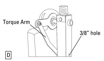
Locate the 3/8'' hole in the display shaft located one foot down from the top and use one  $3/8'' \times 4''$  bolt, two 3/8''washers and 3/8'' nut to secure the torque arm in the lower hole, and tighten.
