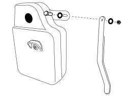
Install the top of the torque arm to the tear drop bracket on the power unit and fasten using the  $3/8'' \times 11/4''$  bolt, 2 flat washers, and 3/8'' lock nut.
