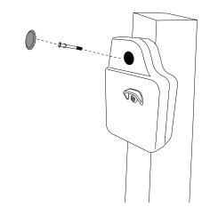
Install 3/8" bolt and washer through drive stub and tighten.
