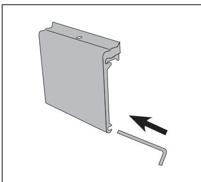
3. Use the hex wrench to tighten the set screw, expanding the hinge bracket down into the lower edge of the groove until it is snug. The accessory mount should now be immobile with both edges seated firmly into the rail track.
