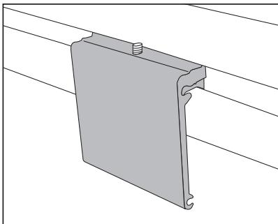
2. Locate the desired position along a SureMount rail track. Place the accessory mount into the rail groove so the lip catches the top edge of the rail track.
