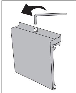
1. Remove the hex wrench from the hex wrench sleeve at the bottom of the accessory mount. Loosen the set screw in the accessory mount to allow the hinge bracket a full range of motion.
