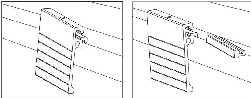
2. Locate the desired position along the rail track. Place the accessory mount into the rail groove so the lip catches the top edge of the rail track.
