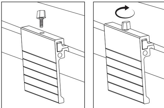
4. Center the slide insert and use the knob screw to tighten the set screw, expanding the hinge bracket down into the lower edge of the groove until it is snug. The accessory mount is now attached to the rail track.
