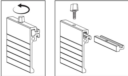
1. Remove the knob screw from accessory mount allowing the slide insert to be removed and the hinge bracket to have a full range of motion when installing.
