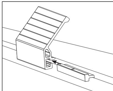
2. Locate the desired position along the rail track. Place the accessory mount into the rail groove so the lip catches the top edge of the rail track.
