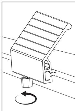
4. Center the slide insert and use the knob screw to tighten the set screw, expanding the hinge bracket down into the lower edge of the groove until it is snug. The accessory mount is now mounted to the rail track.
