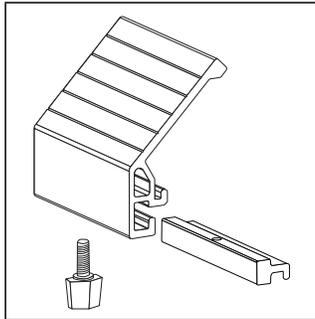
1. Remove the knob screw from accessory mount allowing the slide insert to be removed and the hinge bracket to have a full range of motion when installing.
