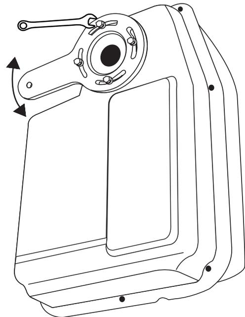
***After all connections use a 10 mm wrench to adjust and straighten if necessary.***
