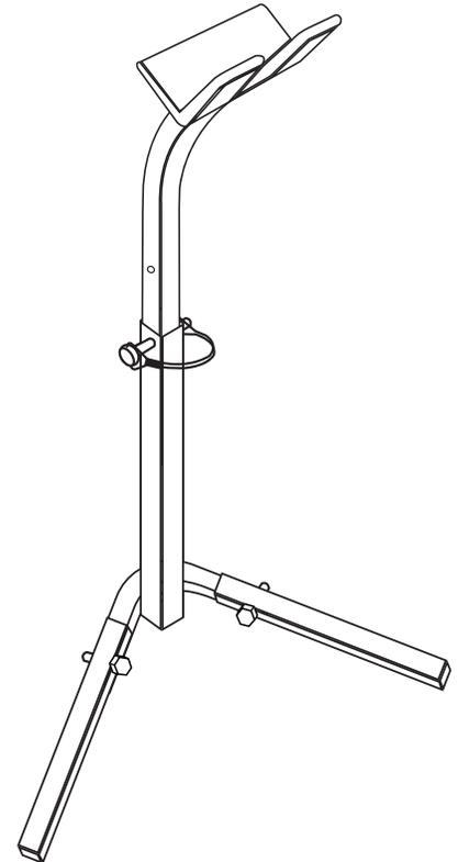
Stand height can be adjusted by removing lynch pin and lifting storage bracket. Always fasten lynch pin securely through center post and storage bracket after height adjustments.
