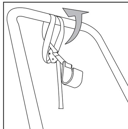
Install the lift strap by wrapping the twisted sewn end of the strap over the handle and drop the cinch buckle through the loop with the hook facing forward.
